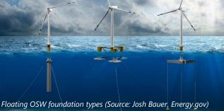
The depth of Maine's coastal waters, which are routinely over 250 feet deep at distances of 10 nautical miles (nm) from the shoreline, rule out the economical use of fixed-bottom foundations.
